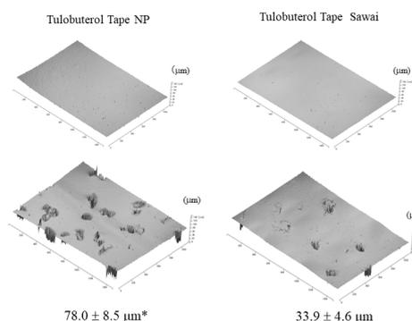
**Figure 4.** Followability test. Tulobuterol Tape Sawai and Tulobuterol Tape NP were placed on sandpapers. 1 min later, the sandpaper was removed to measure the depth of 6 pores with a laser microscope. Values are expressed as mean  $\pm$  SE ( $n = 6$ ).  $p < 0.05$  (Welch's *t*-test). SE, standard error.
