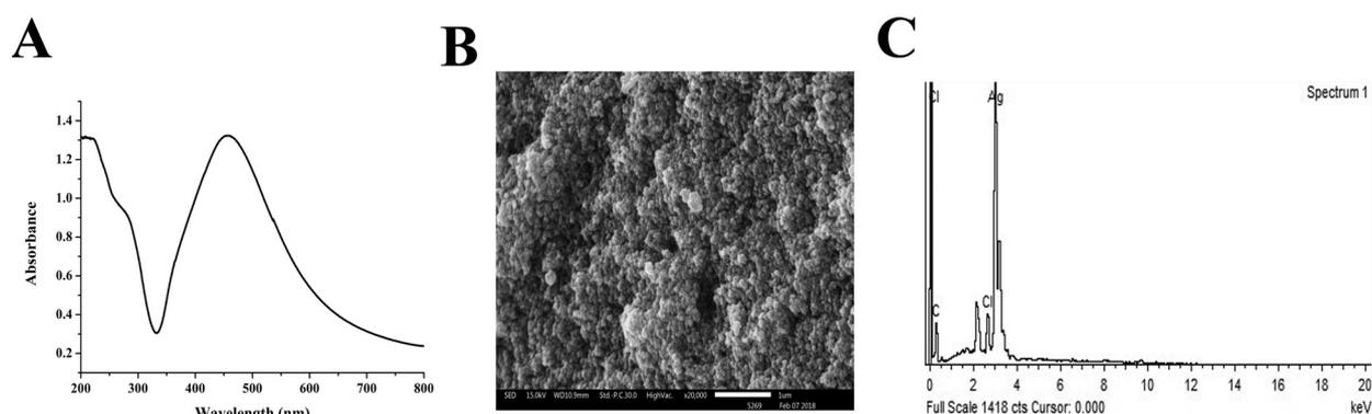
Figure 1. The UV-vis spectrum (A), surface morphology (B), EDX spectrum of Ag signal (C) of AgNPs.
