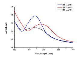
Figure 3. UV-vis spectra of the obtained AgNPs.
