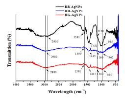
Figure 4. FTIR of the obtained AgNPs.
