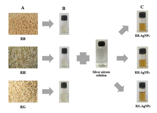
Figure 2. Outer appearance of three parts of rice grains (A), rice extracts (B), and the obtained AgNPs (C).
