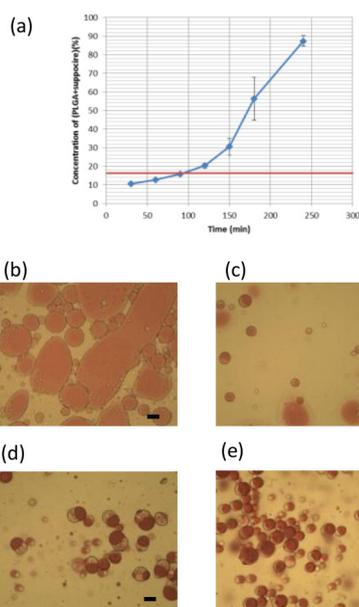
**Figure 6. PLGA-Suppcire<sup>®</sup> AM concentration profile and state of emulsion during solvent evaporation process.** (a) Residual solvent profile during solvent evaporation process. Red line indicates critical concentration of phase separation. The state of emulsion was (b) 60, (c) 90, (d) 150, and (e) 240 min of solvent evaporation time; Ex. 4. Scale bar, 20  $\mu\text{m}$ .
