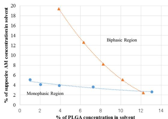
**Figure 3. Phase diagram of poly (lactic-co-glycolic) acid (PLGA)-Suppocire® AM-organic solvent.** Critical line between monophasic and biphasic region, using (▲) methylene chloride and (●) ethyl acetate as organic solvents.
