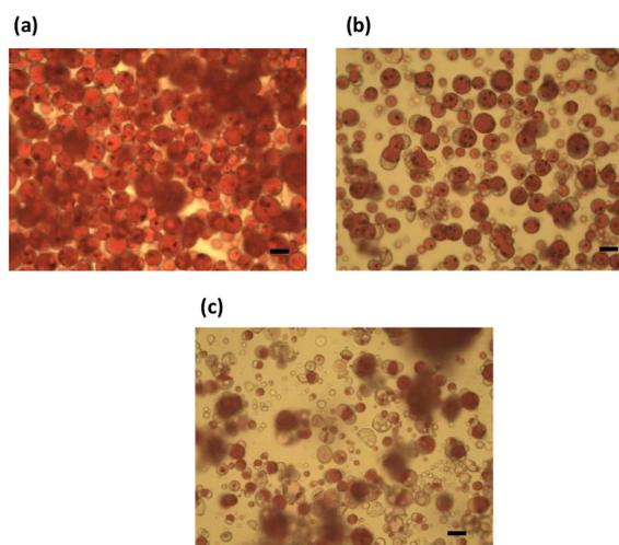
**Figure 7. Effect of addition of aqueous phase after emulsification process on formation of Janus particles.** Optical micrograph of emulsion after 360 min of solvent evaporation process. Addition of (a) 200 mL water (condition A); Ex.7, (b) 100 mL water (condition B); Ex.6, and (c) no water (condition C); Ex.5. Scale bar, 20  $\mu\text{m}$ .
