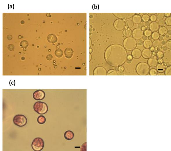
**Figure 4. Optical micrograph of Janus particles.** Janus particles fabricated using (a) methylene chloride; Ex.1 and (b) ethyl acetate; Ex.2 as oil phase solvents. (c) Janus particles fabricated using methylene chloride adding Oil Red O to oil phase solvent; Ex.3. Scale bar, 20  $\mu\text{m}$ .
