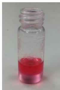
**Figure 5. Partition in phase separated solution of poly (lactic-co-glycolic) acid (PLGA)-Suppcire<sup>®</sup> AM-methylene chloride.** Poly (lactic-co-glycolic) acid (PLGA) and Suppcire AM (200 mg each) were dissolved in 0.3 g 0.02% Oil Red O-methylene chloride, and resultant solution was centrifuged.
