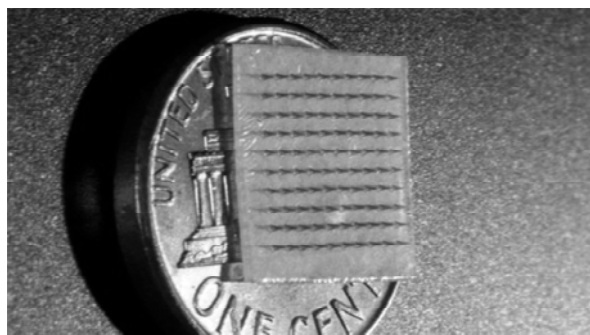
Figure 5. Micromissile capsules, 100 capsules, are formed on 1.0 cm 2 patch.
