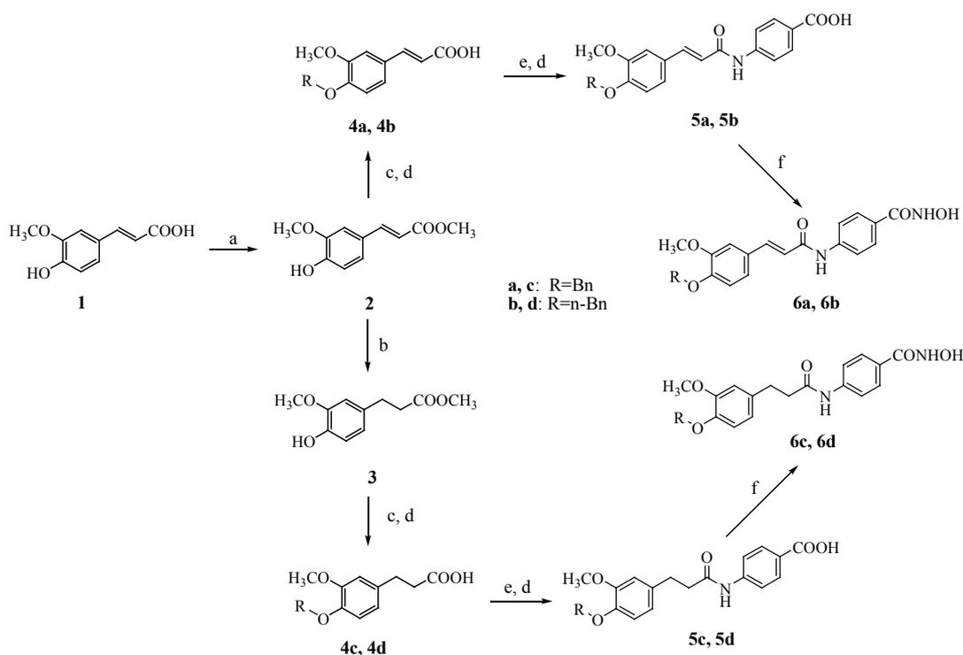
**Scheme 1.** Synthetic scheme, reagents and conditions: (a) PTS, CH<sub>3</sub>OH, 80°C; (b) H<sub>2</sub>, 10% Pd-C, CH<sub>3</sub>OH; (c) RBr, KOH, DMF, r.t.; (d) 2 mol/L NaOH, EtOH, 75°C; (e) SOCl<sub>2</sub>, THF, methyl 4-aminobenzoate; (f) ClCOOBu-*i*, Et<sub>3</sub>N, NH<sub>2</sub>OH·HCl, THF, 0°C.
