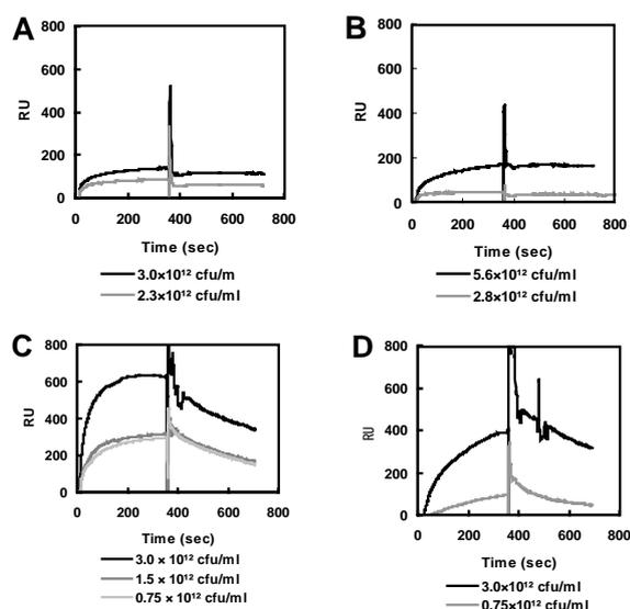
**Figure 3.** SPR analyses of scFv-presenting phage antibodies. Phage antibodies at indicated concentrations were passed over the IGF-IR-immobilized CM3 chip at a flow rate of 5  $\mu$ L/min as described in the Methods. The sensorgrams are 2A1 (A), 3E2 (B), 3H5 (C), and 4C5 (D) phage antibodies, respectively.
