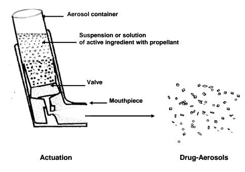
Figure 1. Schematic diagram of aerosol delivery of drugs from pMDI. Modified form Dalby et al. (2).
