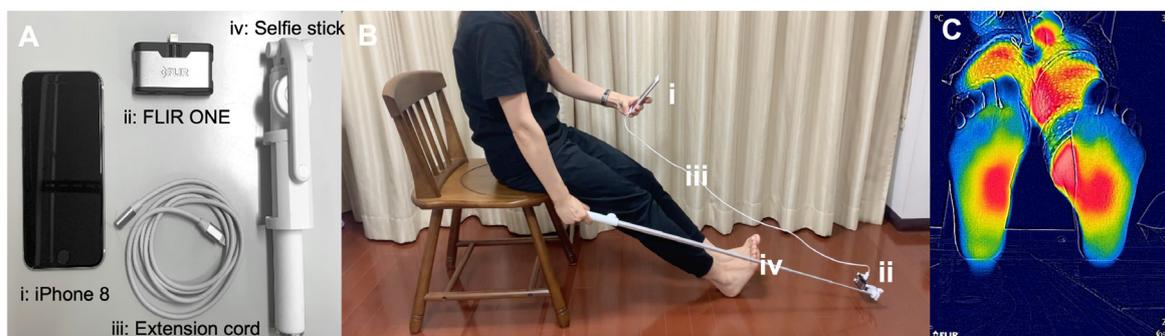
**Figure 1. Demonstration of the use of the self-monitoring thermography set.** The components of the set are shown in picture A, including a smartphone (iPhone 8) (i), a smartphone-based thermography FLIR ONE (ii), an extension cord (iii) to connect the phone and the thermography, and a selfie stick (iv) to control the angle of the thermography. Picture B shows the demonstration of the use of the set, and the taken thermographic image (C).
