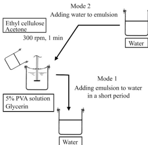
**Figure 1. Illustration of the proposed method for preparing EC microspheres.** In mode 1, the emulsion is added to water instantaneously. In mode 2, water is added to the emulsion for 1 min, 3 min, 5 min, 10 min, or 20 min.
