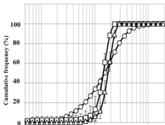
**Figure 3. Weight and size distributions of the fabricated EC microspheres.** ○: proposed method (mode 1), □: conventional O/W-type emulsion solvent evaporation method, △: conventional W/O/W-type emulsion solvent evaporation method. The data shown represent the mean  $\pm$  standard deviation (SD) ( $n = 3$  batches).
