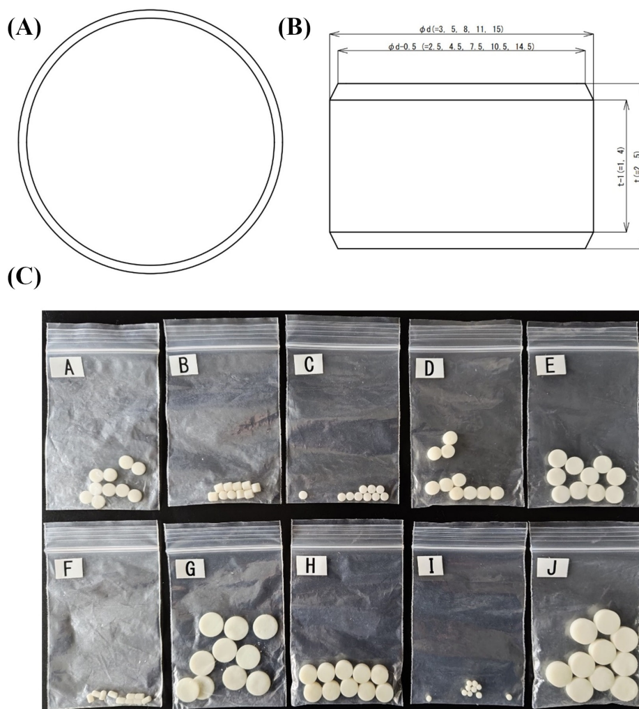
Figure 1. Diagram of dummy tablets produced using a 3D printer. (A) Top view of dummy tablets. (B) Side view of dummy tablets; d: diameter (mm), t: thickness (mm). (C) Tablets and packs were used in the test. A sensory test was conducted in which the tablets were available for visual and tactile examination.
